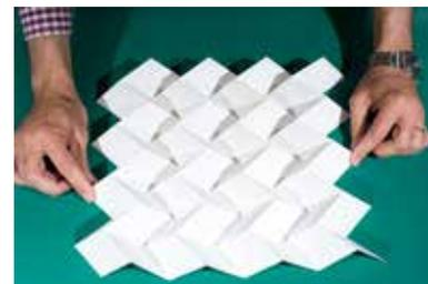
A comparison between the second and third figures shows that the material exhibits a negative Poisson’s ratio – meaning it dilates when stretched.
