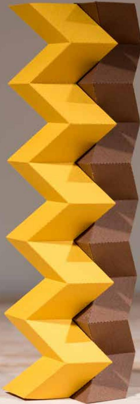
Two structures paired in the "zippered tube" configuration are stiff enough to hold weight, yet can return to their flat states for easy shipping or storage.
