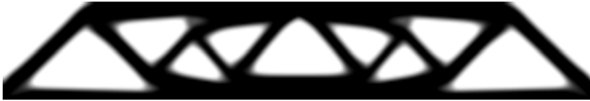
Fig. 6. Final density field for the MBB problem and \beta = 0.06 plotted in grayscale. This result was generated using the TMP algorithm with \tau_0 = 2 and m_n = 1 .
