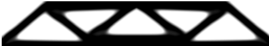
Fig. 10. Final density field for the MBB problem with \beta = 0.06 and subject to volume constraint with \Theta = 0.5 . This result was generated using the FBS algorithm with \tau_0 = 2 .
