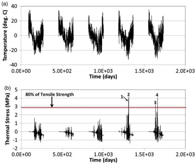
Figure 4. Results from preanalyses. (a) Winter time surface temperatures for five-year analysis period and (b) resulting thermal stresses where four critical events were identified.
