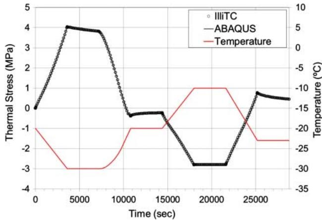
Figure 6. Comparisons for thermo-viscoelastic stress predictions using IlliTC and commercial FE programme ABAQUS.
