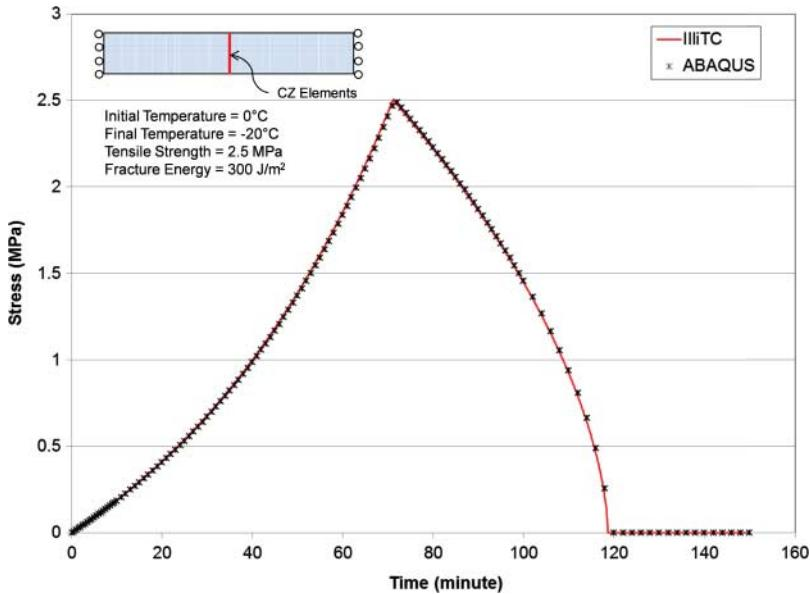
Figure 7. Comparisons of stress for a thermo-viscoelastic body with CZ fracture for predictions using IlliTC and commercial programme ABAQUS.
