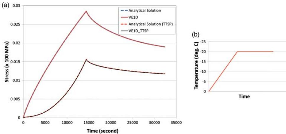
Figure 3. Verification of preanalyser. (a) Comparison of stresses obtained with the preanalyser (VE1D) and the analytical solution and (b) thermal loading.
