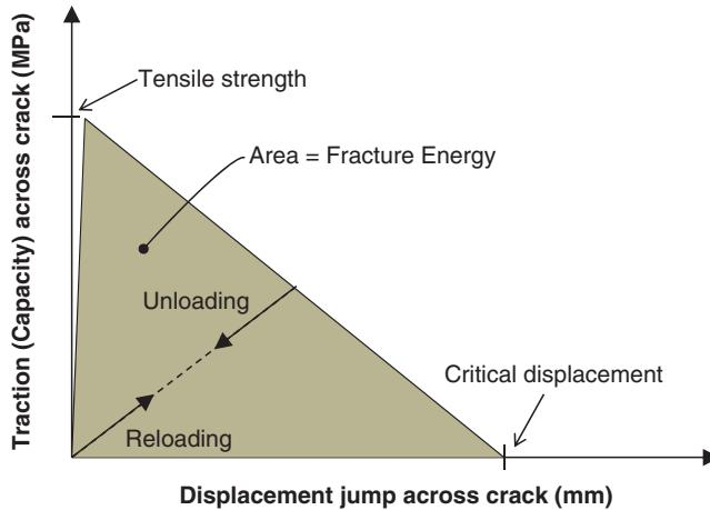
Figure 5. Bi-linear CZM used in IlliTC.
