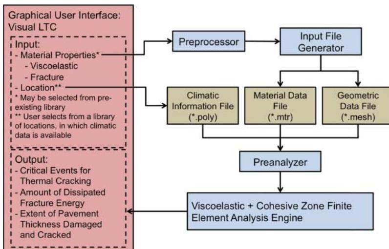
Figure 1. Flowchart of new TCMModel – IlliTC.
