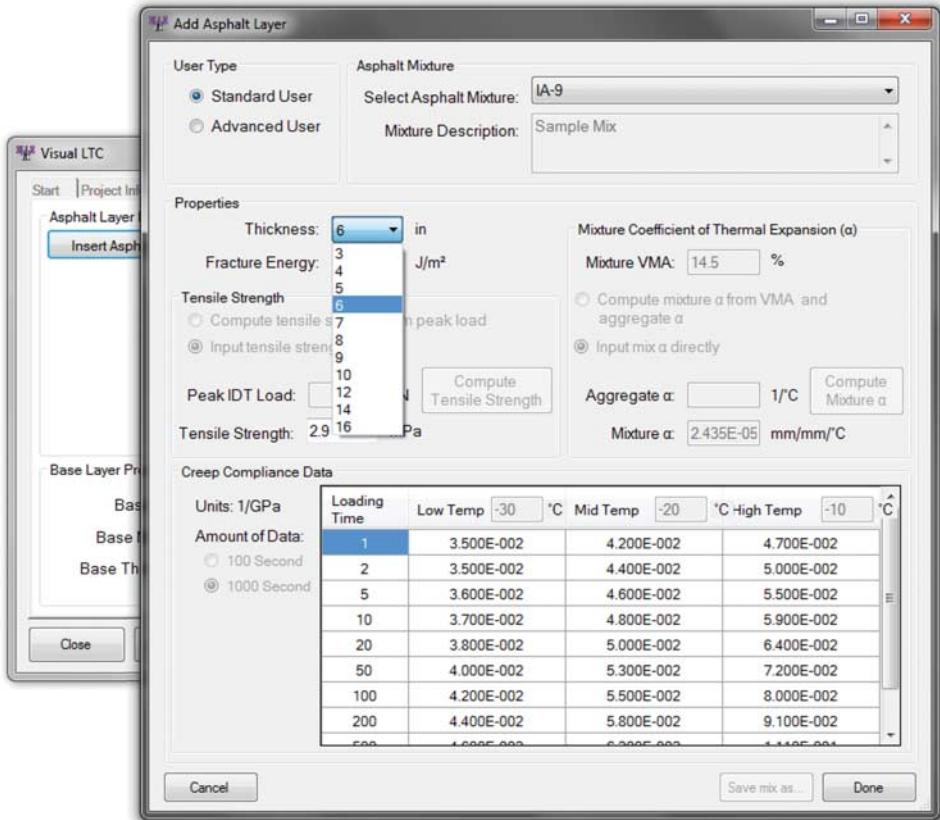
Figure 2. Visual LTC window – asphalt layer material properties.
