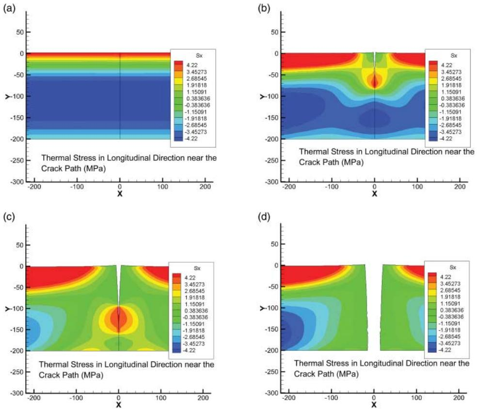
Figure 9. Results from FEA for MnROAD section 19 (calibration field section) (tensile strength = 4.22 MPa). (a) Thermal stress built-up along longitudinal direction (surface temperature =  $-23.3^{\circ}\text{C}$ ), (b) partial depth softening damage (surface temperature =  $-24.3^{\circ}\text{C}$ ), (c) partial depth crack (surface temperature =  $-25.4^{\circ}\text{C}$ ), and (d) fully formed crack (surface temperature =  $-29.6^{\circ}\text{C}$ ).
