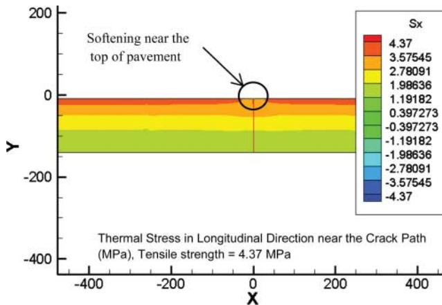
Figure 11. Thermal stresses at the end of the critical event for validation section 4.
