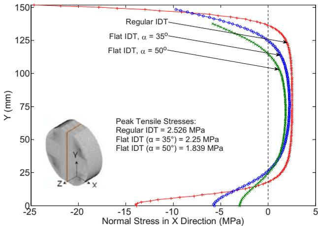
FIG. 11—Normal stress in the X direction, Mix-40.
