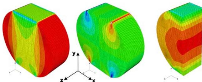
FIG. 7—Normal stress in the  $Y$  direction, shear stress in the  $XY$  plane, and normal stress in the  $X$  direction.
