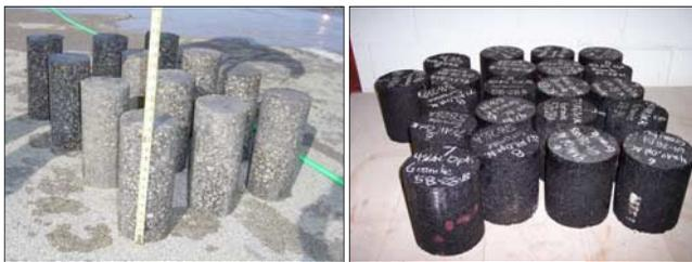
FIG. 2—Field samples (left) and laboratory samples (right); both sets of these samples are 150 mm diameter samples of asphalt concrete.
