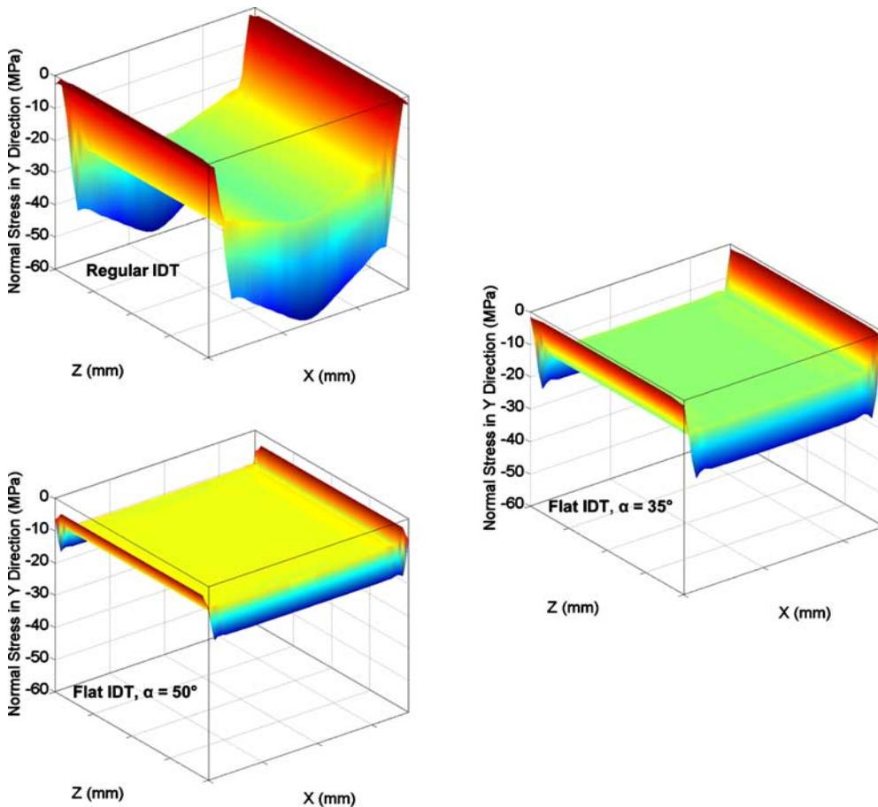
FIG. 10—Three-dimensional peak normal stresses in the Y direction, Mix-40.
