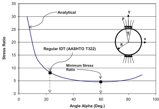
FIG. 6—Compressive/tensile stress ratio versus internal angle  $\alpha$  (elastic Hon-dros solution).
