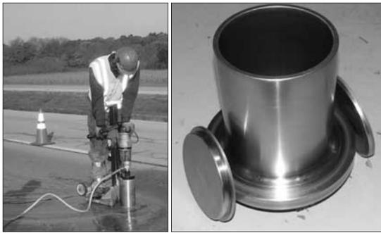
FIG. 1—Field sample extraction (left) and laboratory mold (right, from Ref 1); both fabrication methods produce 150 mm diameter samples of asphalt concrete.
