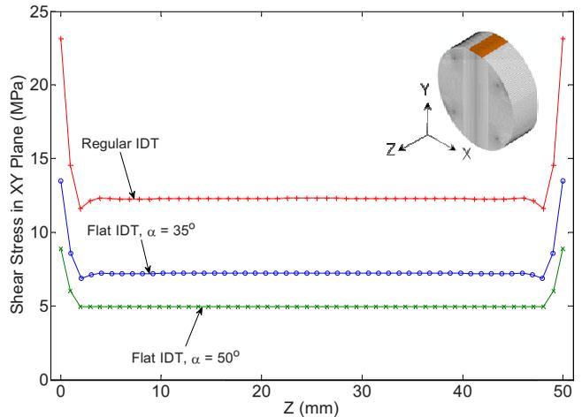
FIG. 12—Peak shear stresses in the XY plane, Mix-40.
