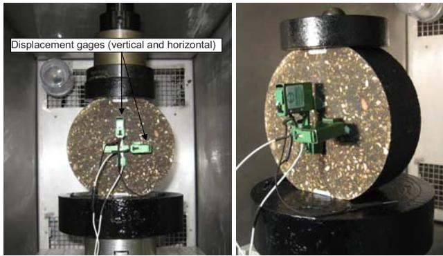
FIG. 13—Flattened IDT test setup.
