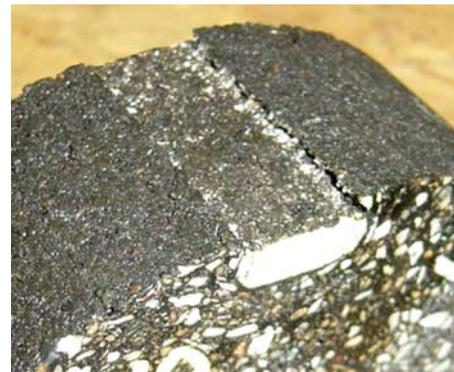
FIG. 4—Undesirable crushing failure under regular IDT loading head (Mix-40).
