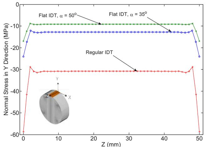
FIG. 9—Peak normal stresses in the  $Y$  direction, Mix-40.
