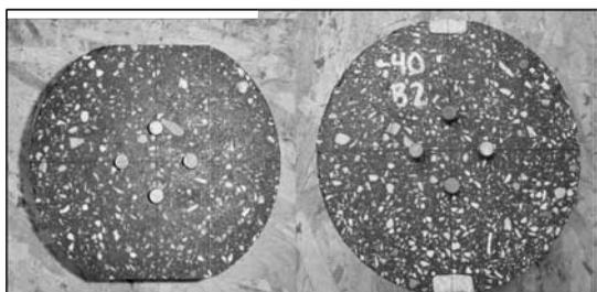
FIG. 14—Flattened (left,  $\alpha = 50^\circ$ ) and regular (right) IDT test specimens.
