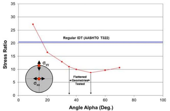
FIG. 8—Compressive/tensile stress ratio versus angle  $\alpha$  from FE analysis.
