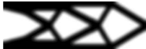
**a** FE mesh size 240x80, element-based approach with Q4 elements ( $C=210.68$ )
