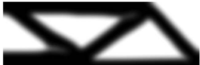
**c** Mesh resolution: 150x50 Q4/Q4M elements
