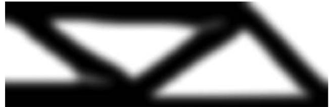
**b** Mesh resolution: 90x30 Q4/Q4M elements
