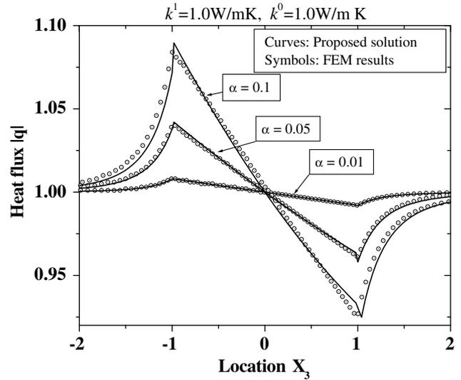
Fig. 5. Effect of matrix material gradation on the heat flux distribution along the  $x_3$  axis.
