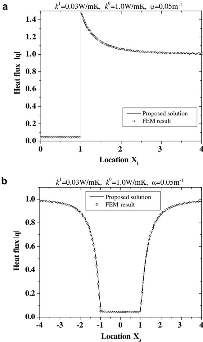
Fig. 4. Comparison of heat flux distribution for an air void embedded in a graded material for the proposed solution and the finite element result: (a) along the  $x_1$  axis and (b) along the  $x_3$  axis.
