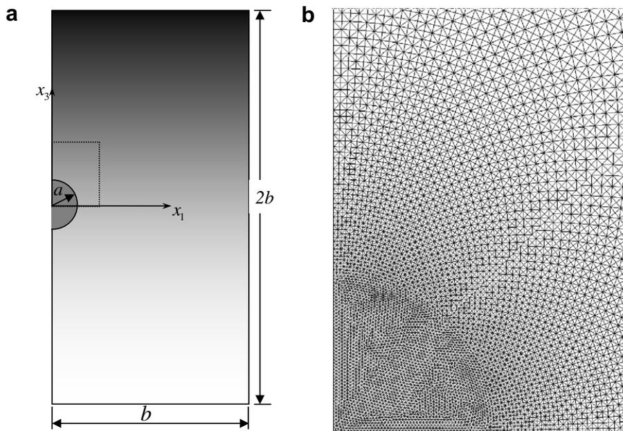
Fig. 3. Finite element model for a single inhomogeneity embedded in a large functionally graded material: (a) axisymmetric geometry, and (b) finite element mesh in the dotted line box.
