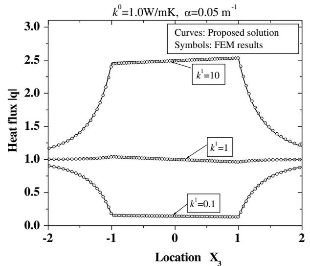
Fig. 6. Effect of the particle's thermal conductivities on the heat flux distribution along the  $x_3$  axis.
