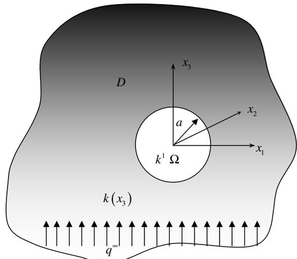
Fig. 2. A single spherical inhomogeneity in an FGM matrix subjected to a uniform heat flux field.
