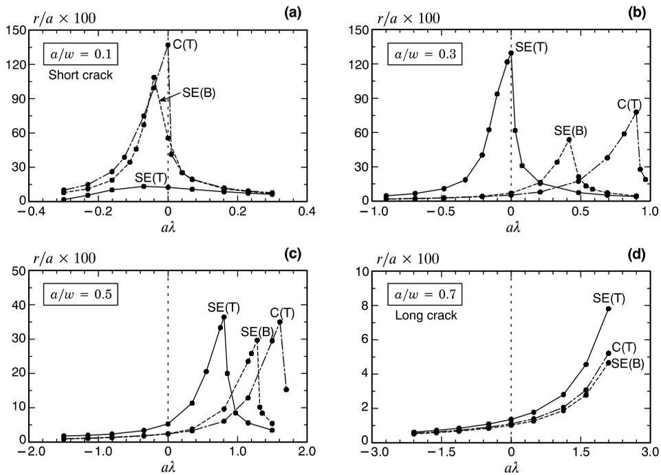
Fig. 4. Extent of  $K$ -dominance for SE(T), SE(B) and C(T) specimens considering material gradation and crack geometry.
