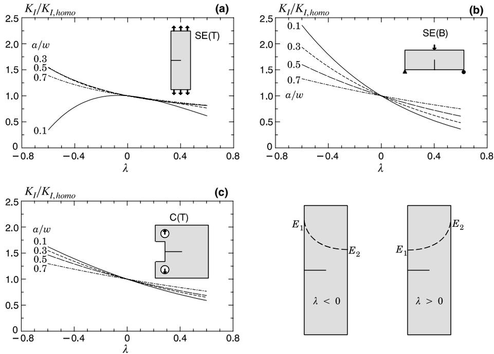
Fig. 3. Effect of material gradation on  $K_I$  for SE(T), SE(B) and C(T) specimens with various crack lengths.
