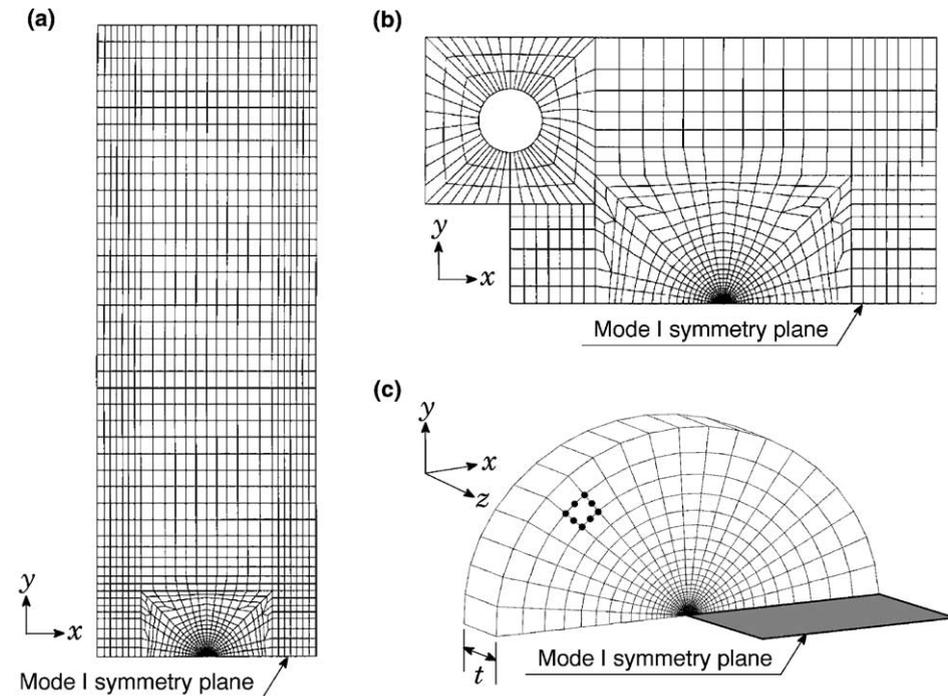
Fig. 2. Typical finite element meshes used in the present study: (a) SE(T) and SE(B); (b) C(T); (c) close-up view of the circular domain (67 rings) at the crack-tip.
