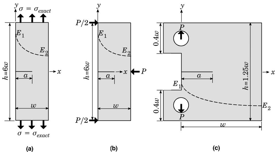
Fig. 1. Fracture specimens considered in the present study: (a) single-edged tension, SE(T); (b) single-edged bending, SE(B); (c) compact tension, C(T). Note that the specimen thickness  $t = 0.01w$  for all specimens. Material properties are graded in the  $x$ -direction.
