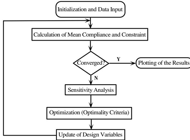
Fig. 1: Flow Chart of Optimization Procedure.
