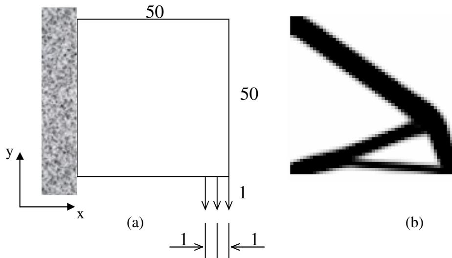
Fig. 2: (a) Initial domain discretized with a 50 x 50 mesh; (b) Topology for comparison obtained considering SIMP model for homogeneous material ( $\alpha=\beta=0$ ) with 30% volume constraint and filtering (radius equal to 1.5).
