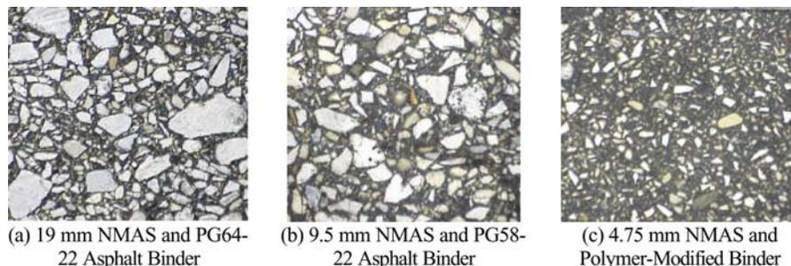
FIG. 4—Asphalt concrete mixtures with nominal maximum aggregate size (NMAS) and asphalt binder type.
