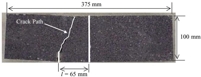
FIG. 10—Mixed-mode fracture test using the offset notch method ( $a/W = 0.19$ ).
