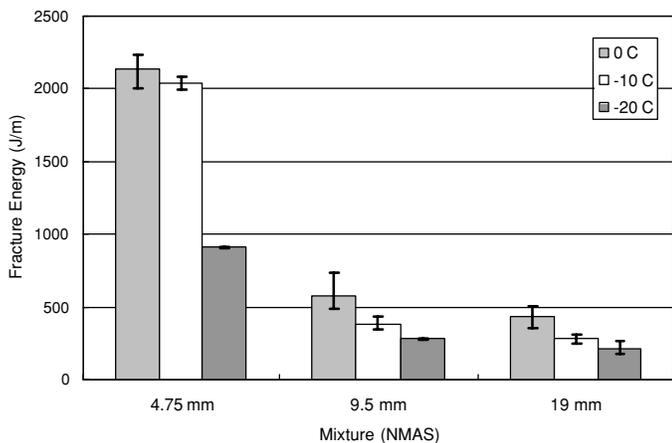
FIG. 8—Average fracture energy for each mixture and temperature with minimum and maximum deviation from the average.
