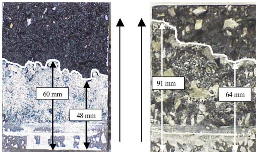
FIG. 6—Crack-front profile using dye penetration for 4.75 mm NMAS (left) and 9.5 mm (right) mixtures.
