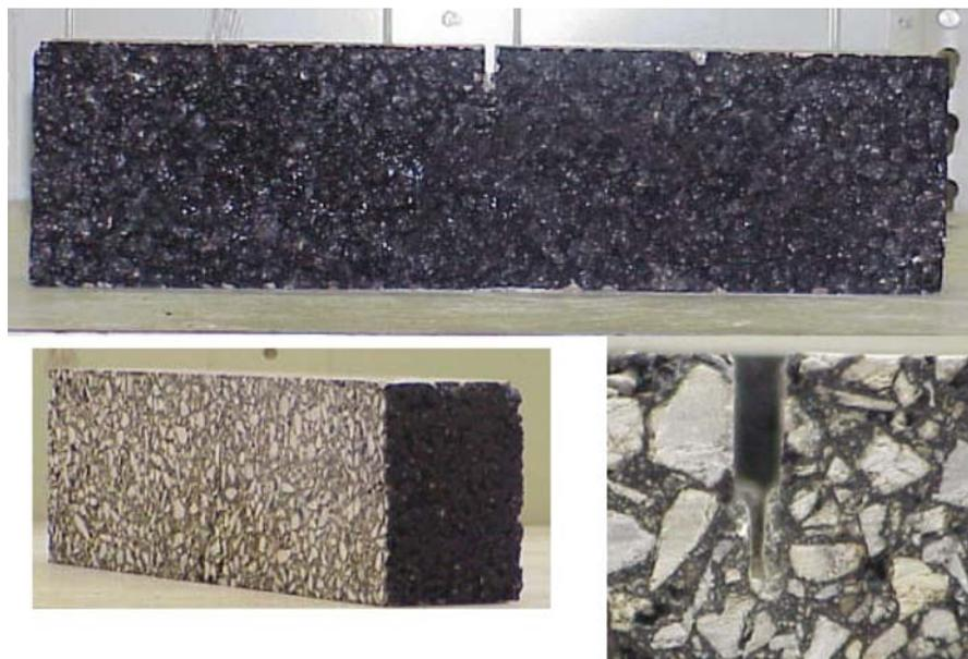
FIG. 1—Final SE(B) specimen with mechanical notch.
