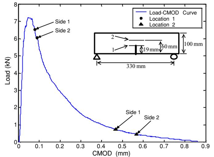
FIG. 5—Load versus CMOD with crack detection gages.
