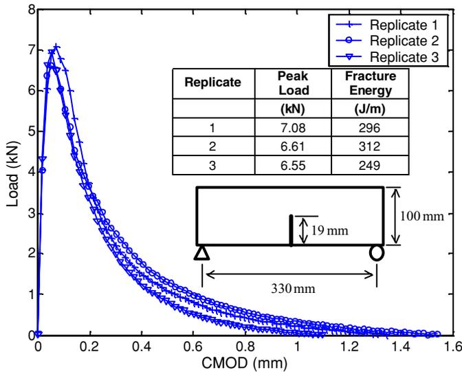
FIG. 7—Load-CMOD curves for three replicates of the 19 mm NMAS mixture at  $-10^{\circ}\text{C}$ .
