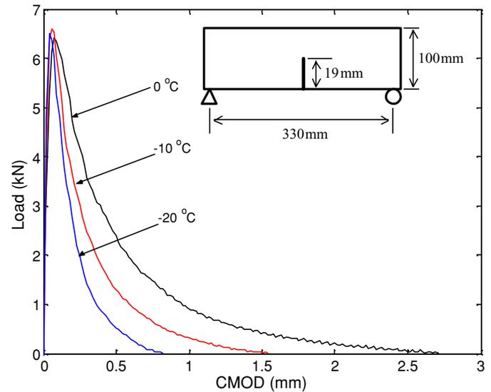
FIG. 9—Load-CMOD curves for the 19 mm NMAS mixture at three temperatures:  $-20^{\circ}\text{C}$ ,  $-10^{\circ}\text{C}$ , and  $0^{\circ}\text{C}$ .
