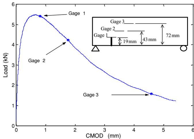
FIG. 11—Load-CMOD for mixed-mode fracture test with crack detection gages at 19, 43, and 72 mm from the bottom of the beam.
