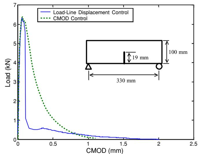
FIG. 3—Difference between load-line displacement and CMOD control methods (tests conducted at  $-10^\circ\text{C}$ ).
