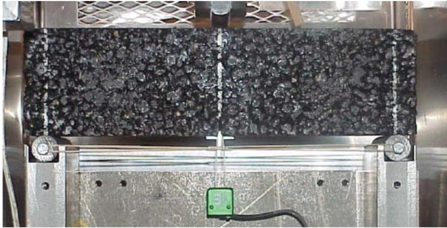
FIG. 2—SE(B) test fixture and clip gage.
