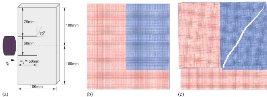
Figure 9. Simulation of the Kalthoff and Winkler [31] experiment in which a pre-cracked is subjected to an impact by a projectile [8]: (a) actual experimental configuration; (b) original mesh employing symmetry; and (c) deformed mesh illustrating spontaneous mixed-mode crack propagation.
