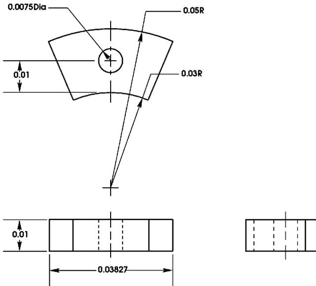
Fig. 4 Geometry of the functionally graded rotor
