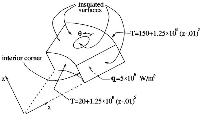
Fig. 5 Thermal boundary conditions on the rotor
