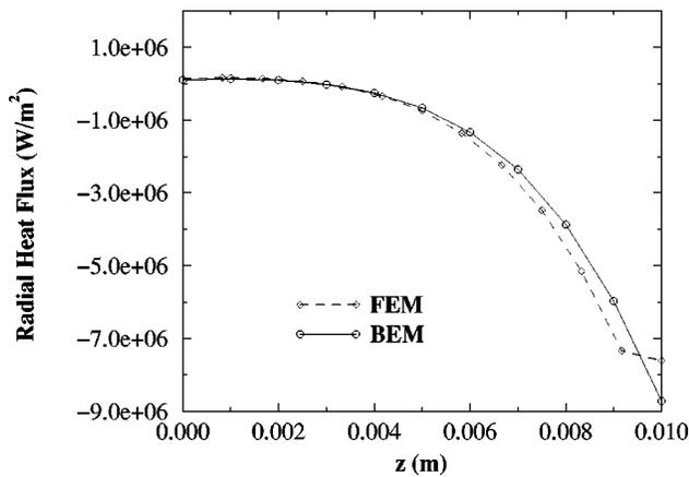
Fig. 9 Radial heat flux along the inside corner
