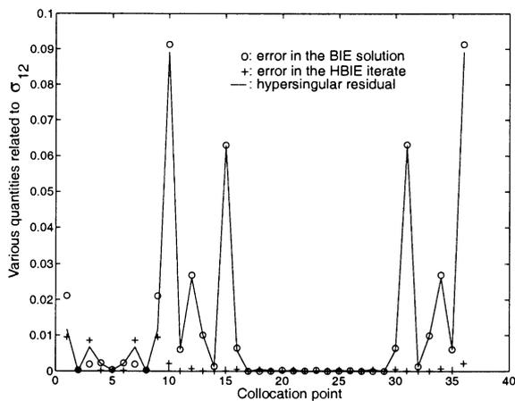
Fig. 4. Absolute values of error in the BIE solution, error in the HBIE iterate, and the hypersingular residual, for  $\sigma_{12}$ . All variables are unscaled.
