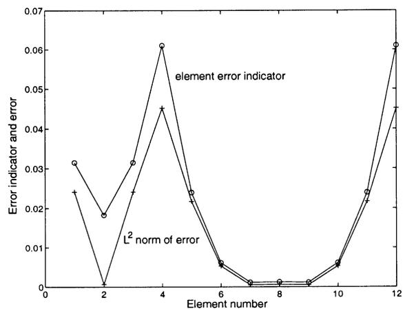
Fig. 6. Stress residual based element error indicator compared with error in boundary stresses.
