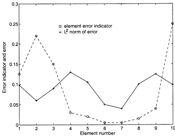
Fig. 8. Traction residual based element error indicator compared with error in the unspecified boundary data.
