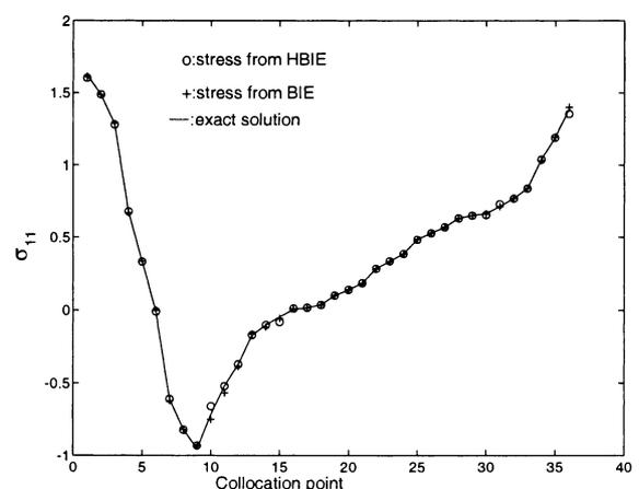
Fig. 2. Comparison of analytical and numerical solutions for  $\sigma_{11}$ .
