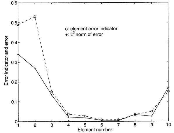
Fig. 9. Stress residual based element error indicator compared with error in boundary stresses.
