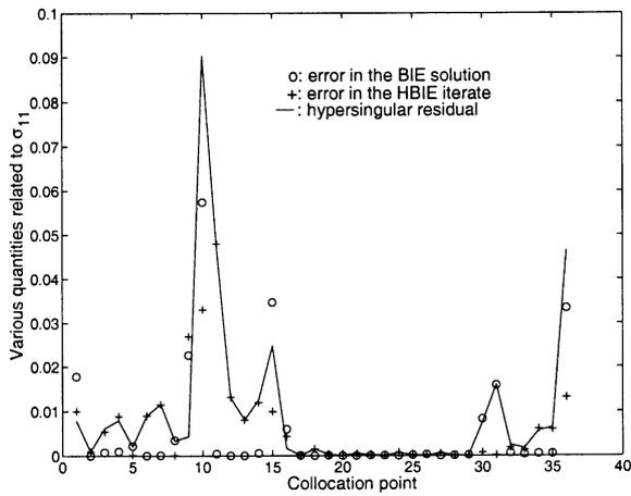
Fig. 3. Absolute values of error in the BIE solution, error in the HBIE iterate, and the hypersingular residual, for  $\sigma_{11}$ . All variables are unscaled.
