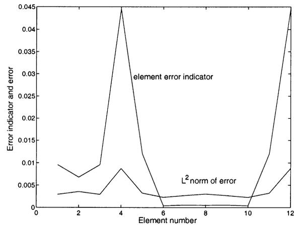
Fig. 5. Traction residual based element error indicator compared with error in the unspecified boundary data.
