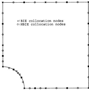
Fig. 7. Discretized domain for the problem of a plate with a hole with 10 elements. Plate side = 4 units, holeradius = 1 unit of length.
