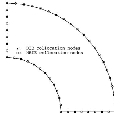
Fig. 1. Discretized domain for the Lamé problem with 12 elements.
