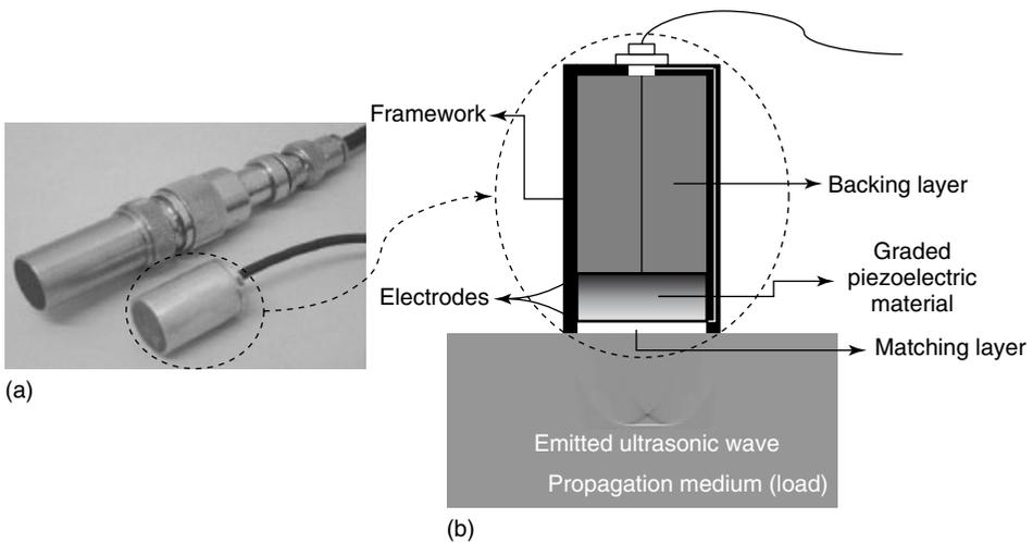
**Figure 8.5** FGM concept applied to piezoelectric ultrasonic transducers: (a) photograph of a typical assembly of an ultrasonic transducer and (b) sketch of the same transducer considering a graded piezoelectric material.
