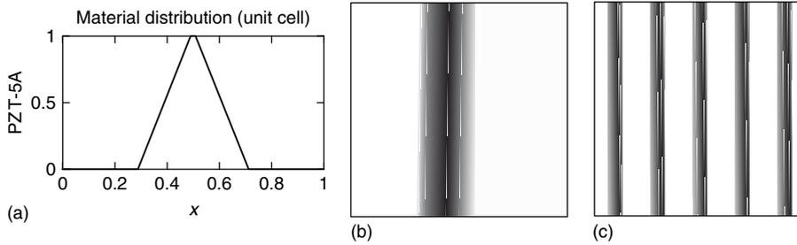
**Figure 8.20** Linear FGM 2-2 piezocomposite. (a) Material distribution graphic of PZT-5A; (b) unit cell; and (c) periodic array.
