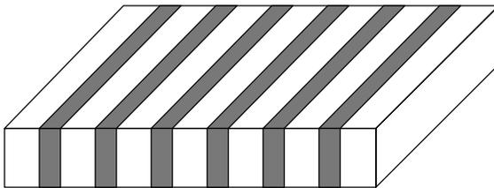
Figure 8.18 2–2 piezocomposite.
