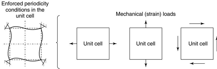
Figure 8.16 Load cases for homogenization of elastic materials.
