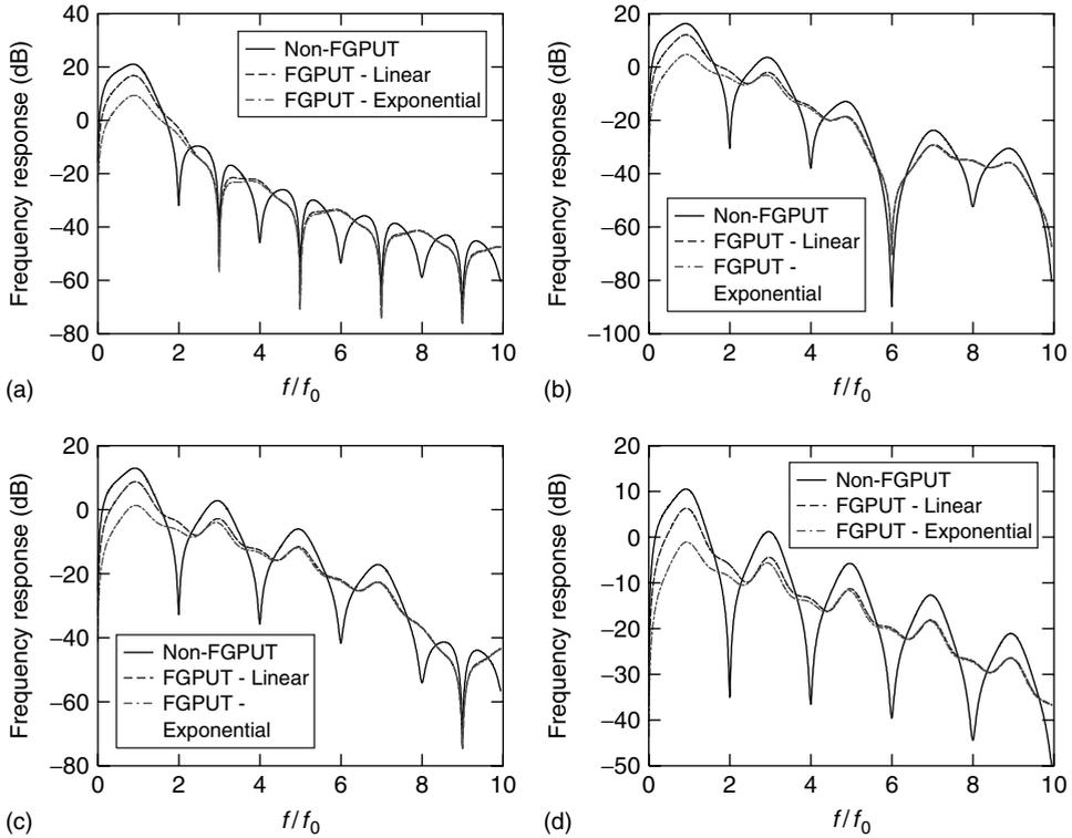
**Figure 8.9** Spectrum of output signals for non-FGPUT and FGPUT systems considering several input excitations: (a) at  $f_0$ ; (b) at  $2f_0$ ; (c) at  $3f_0$ ; and (d) at  $4f_0$ .
