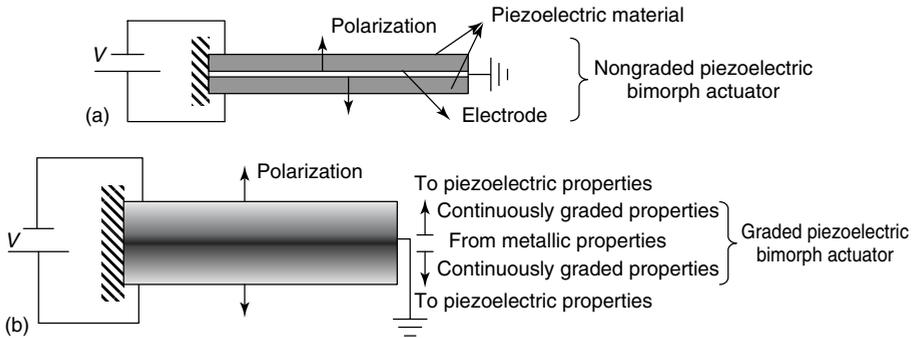
**Figure 8.4** FGM concept applying to bimorph transducers: (a) nongraded piezoelectric transducer and (b) graded transducer from electrode (metallic) properties in the middle to piezoelectric properties on the top and bottom surfaces.
