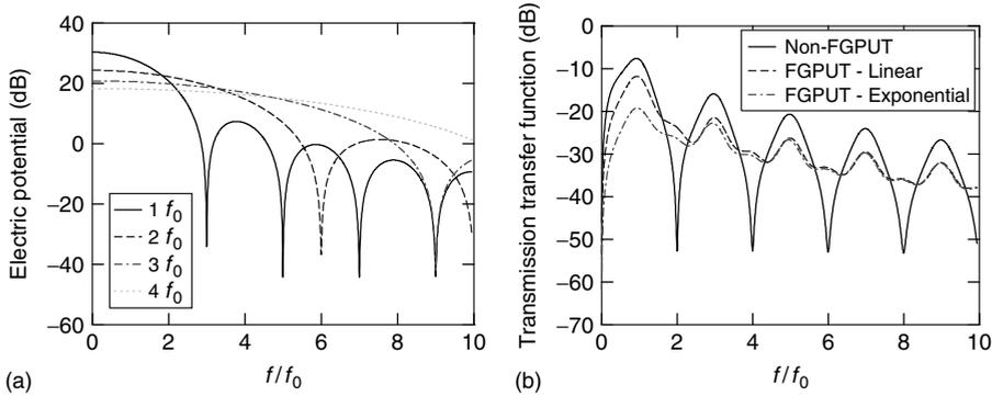
**Figure 8.8** (a) Spectrum of several electrical input excitations (each with different fundamental frequency) and (b) normalized-frequency transmission transfer function (TTF) for both non-FGPUT and FGPUT with linear and exponential gradation functions [30].
