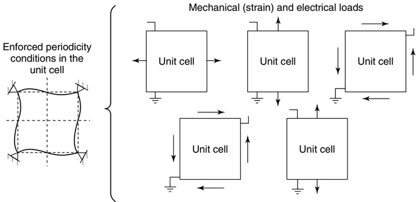
Figure 8.17 Load cases for homogenization of piezoelectric materials.
